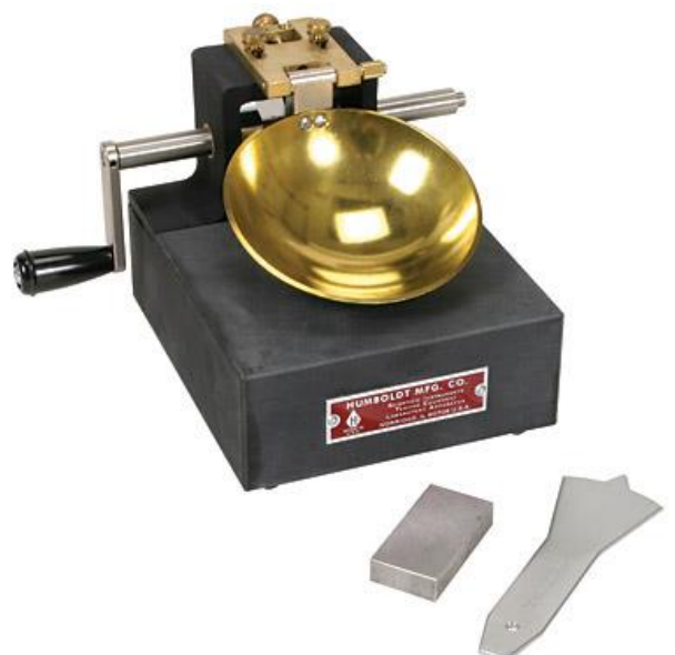
Liquid limit test: (a) liquid limit device; (b) flat grooving tool; (c) wedge grooving tool; (d) soil pat before test; (e) soil pat after test
